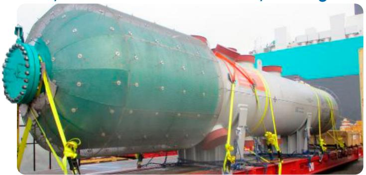
Livo Logistics executed the time sensitive transport of two heavy and oversized boilers, each weighing 87tn and measuring 15.1 x 3.3 x 3.4m. They were transported from Lohfelden to FOB at Bremerhaven Port in Germany including reloading from trucks onto roll trailers as well as full lashing and securing.
