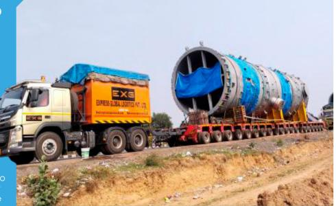
During the arduous journey, the height of the cargo also required the structure of a toll plaza be dismantled and rebuilt for the cargo to pass.
