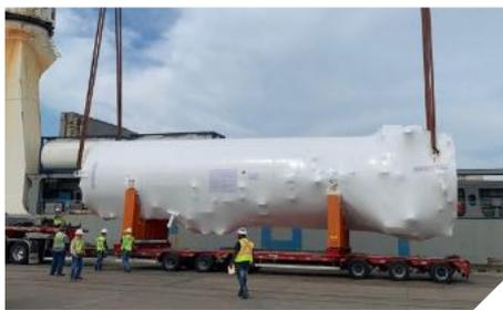
C.H. Robinson Project Logistics helped transport 2,000cbm of LNG equipment from China to Texas for a chemical plant expansion. The project involved a part charter and approximately 65 domestic truck loads, including breakbulk pieces, containers, crates and loose items. The largest piece was a H2 liquefier cold box which weighed 86.82mtn and measured 18.52 x 4.70 x 4.85m.
