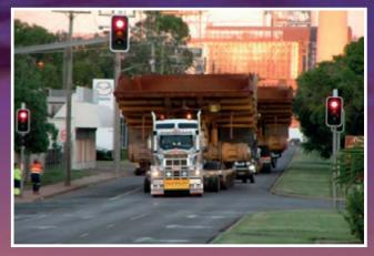
For details and hyperlinks of recent project work handled by Freightplus, including the above photographed movement of 12 CAT789's (each one weighing 142tn and measuring 13.0 x 7.7 x 5.5m) from a mine site in the Australian outback to the Port of Townsville before continuing on to another remote mine site in Indonesia, please visit the online story.
