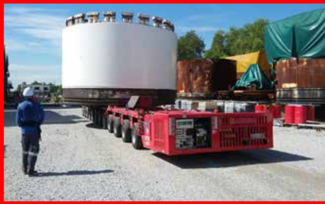
Cargo: Front Shield of Tunnel Boring Machine Dimension: L6.74 m x W6.63 m x H3.80 m Weight: 155 tons Scope: Internal shuttling and lifting
