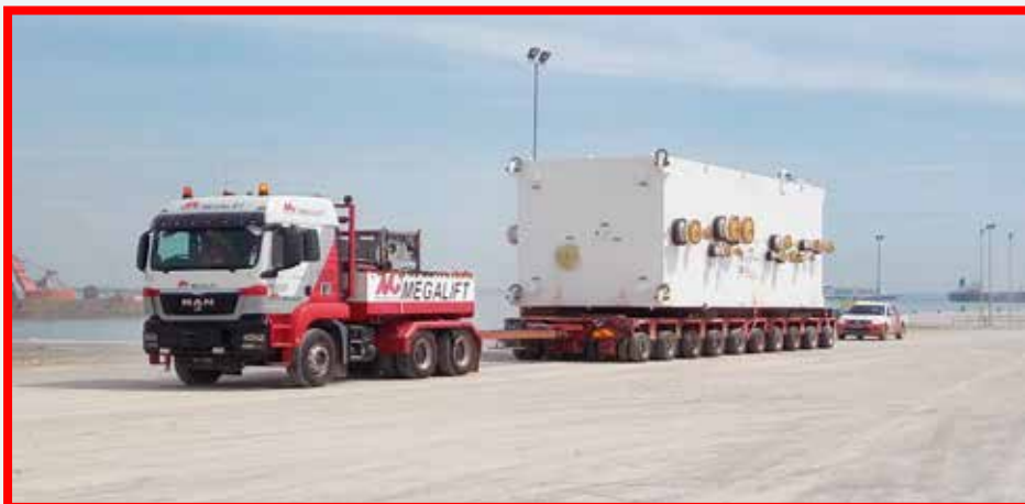
Cargo: ROG Cold Box Dimension: L12.50 m x W4.88 m x H4.42 m Weight: 61.87 tons
