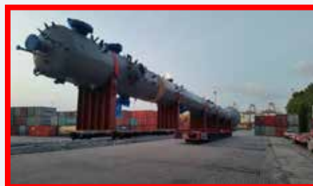
Cargo: Benzene Tower Dimension: L52.55 m x W4.50 m x H5.014 m Weight: 98 tons
