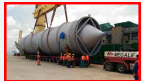
Cargo: Spent Catalyst Hopper Dimension: L33.88 m x W6.12 m x H6.27 m Weight: 160 tons
