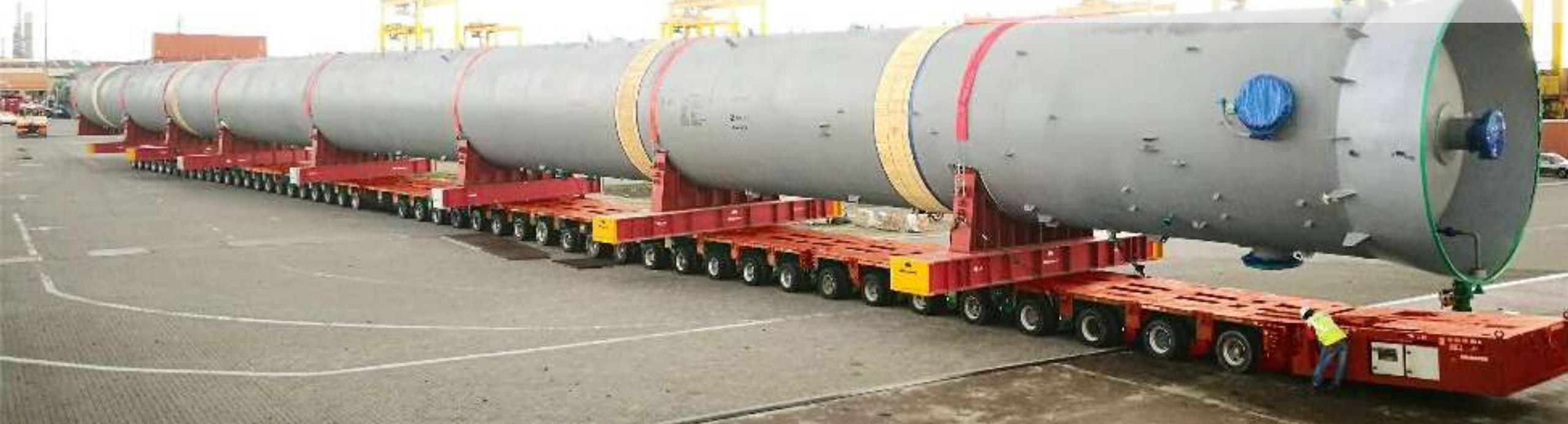
Lotte Chemical TE3 PROJECT (GS Engineering) Year 2016, Sept 5th Propylene Splitter 94m x 5.78m x 5.05m – 580 ton
