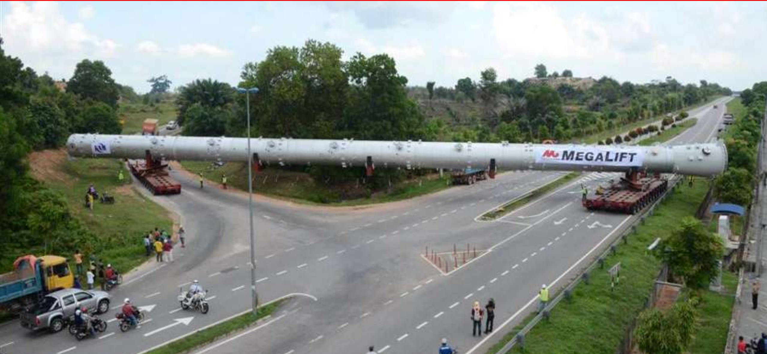
Lanxess Singapore Project (Year 2012) Reactor Column (80m x 6m x 5m – 248 ton)
